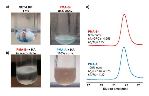
**Figure 1.** Visualization of the heterogeneous nature of (a) SET-LRP of MA in an acetone/water mixture (8/2, v/v) using non-activated Cu(0) wire/TREN/Cu(II)Br<sub>2</sub> as a catalytic system ([MA]<sub>0</sub>/[MBP]<sub>0</sub>/[TREN]<sub>0</sub>/[Cu(II)Br<sub>2</sub>]<sub>0</sub> = 50/1/0.1) and (b) esterification of KA with PMA-Br in acetonitrile. (c) GPC chromatograms of PMA-Br and PMA-A.
