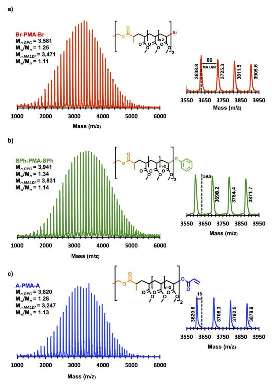
**Figure. 8.** MALDI-TOF of (a) Br-PMA-Br isolated at 93% conversion  $([MA]_0/[BPE]_0/[TREN]_0/[CuBr2]_0 = 50/1/0.4/0.2)$  from SET-LRP of MA in acetone/water (8/2, v/v) mixtures initiated with BPE and catalyzed by non-activated Cu(0) wire at 25 °C, (b) Br-PMA-Br after thio-bromo "click" reaction and (c) A-PMA-A synthesized by esterification of Br-PMA-Br with KA in acetonitrile at 75 °C.
