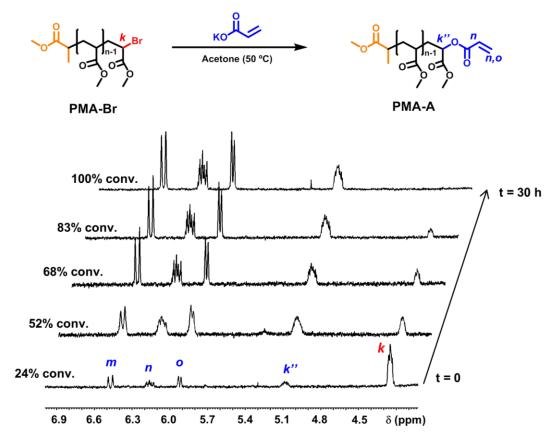
**Figure. 3.** <sup>1</sup>H-NMR evolution traces for the biphasic functionalization of PMA macromonomer  $(M_n = 4,596 \text{ g/mol})$  with KA in acetonitrile. Degree of esterification is shown at the left side of <sup>1</sup>H NMR traces.
