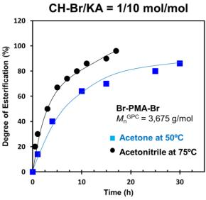
**Figure 6.** Kinetics plots, conversion for the esterification vs time of Br-PMA-Br with KA. Br-PMA-Br isolated at 93% conv. ([MA]<sub>0</sub>/[BPE]<sub>0</sub>/[TREN]<sub>0</sub>/[CuBr<sub>2</sub>]<sub>0</sub> = 30/1/0.4/0.2) from biphasic SET-LRP of MA in acetone/water (8/2, v/v) mixtures initiated with MBP and catalyzed by non-
