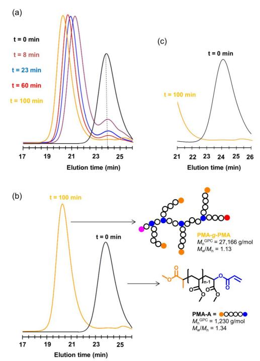
**Figure. 9** (a) GPC evolution and (b,c) initial and final GPC curves for the Cu(0) wire-catalyzed SET-LRP copolymerization of MA with PMA-A macromonomer in an acetone/water (8/2, v/v) mixture initiated with MBP. Reaction conditions:  $[MA]_0/[PMA-A]_0/[MBP]_0/[TREN]_0/[CuBr_2]_0 = 333/5/1/0.4/0.2$ , MA=2 mL, PMA-acrylate = 0.4 g, acetone + water = 0.5 mL, 12.5 cm of 20 gauge Cu(0) wire.
