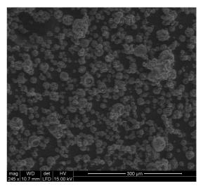
Figure 2. Environmental scanning electron microscope micrograh of thyme oil microcapsules produced with wall material maltodextrin:thyme essential oil load rate of 4:1 at magnification of  $245 \times$ .
