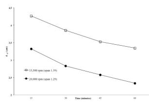
Figure 1. Oil droplet size as d<sub>12</sub> evolution with the time of speed for the production of thyme essential oil O/W emulsion.
