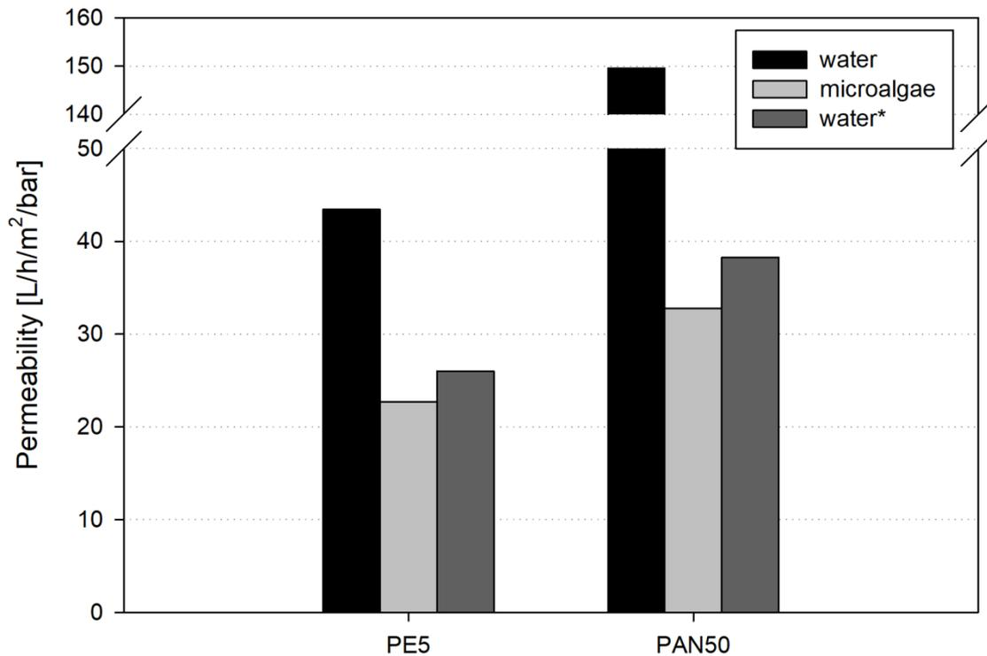
Figure 4: Permeability results for experiments of maximum concentration of *Dunaliella tertiolecta*: water permeability with the virgin membrane, microalgae culture permeability and water\* permeability after the experiment and with the cleaning procedure performed ( $n = 1$ ). PE5 - commercial polyethersulfone membrane, PAN50 – commercial polyacrylonitrile membrane.
