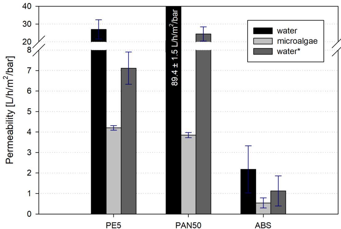
Figure2: Permeability results for the cross-flow filtration of *Dunaliella tertiolecta*: water permeability with the virgin membrane, microalgae culture permeability and water\* permeability after the experiment and with the cleaning procedure performed ( $n = 2$ ). The error bars report standard deviation between measurements. PE5- commercial polyethersulfone membrane, PAN50 – commercial polyacrylonitrile membrane, ABS – own-made acrylonitrile butadiene styrene membrane.
