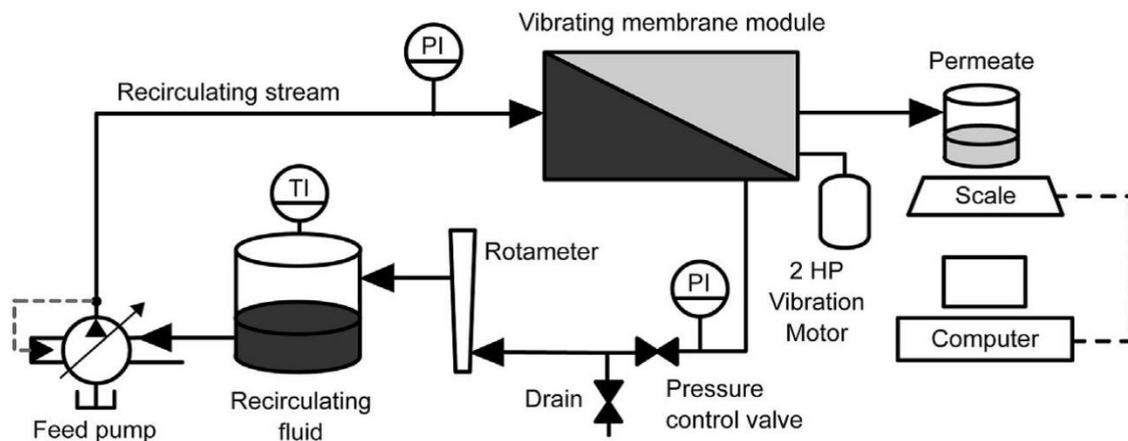
Figure 1: Filtration setups: a) cross-flow filtration; b) dynamic filtration (PI: Pressure Indicator, TIC: Temperature Indicator Controller, TI: Temperature Indicator, HP: Horsepower, SEPA CF2: commercial name for the tangential cross-flow membrane module). [22]
