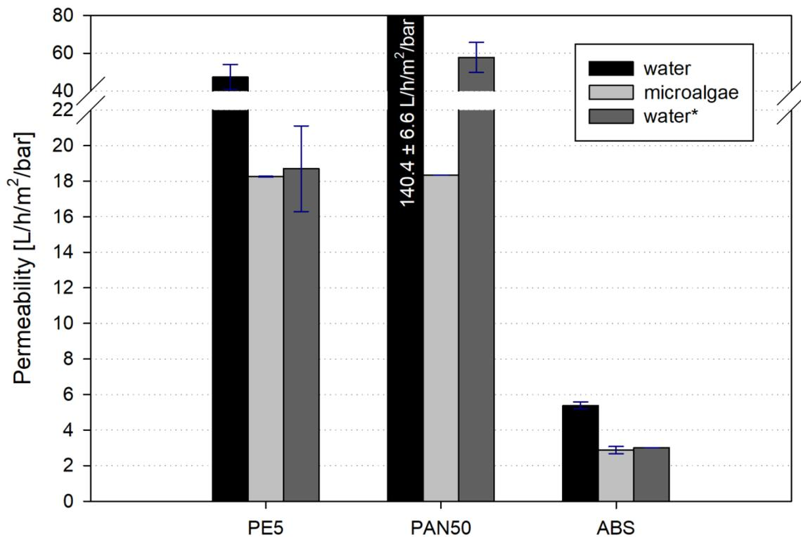
Figure 3: Permeability results for the dynamic filtration of *Dunaliella tertiolecta*: water permeability with the virgin membrane, microalgae culture permeability and water\* permeability after the experiment and with the cleaning procedure performed ( $n = 2$ ). The error bars report standard deviation between measurements. PE5- commercial polyethersulfone membrane, PAN50 – commercial polyacrylonitrile membrane, ABS – own-made acrylonitrile butadiene styrene membrane.
