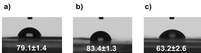
**Figure SI.4.** Water contact angle images of starting polymers a) PEAU, b) PHU and c) PCL.
