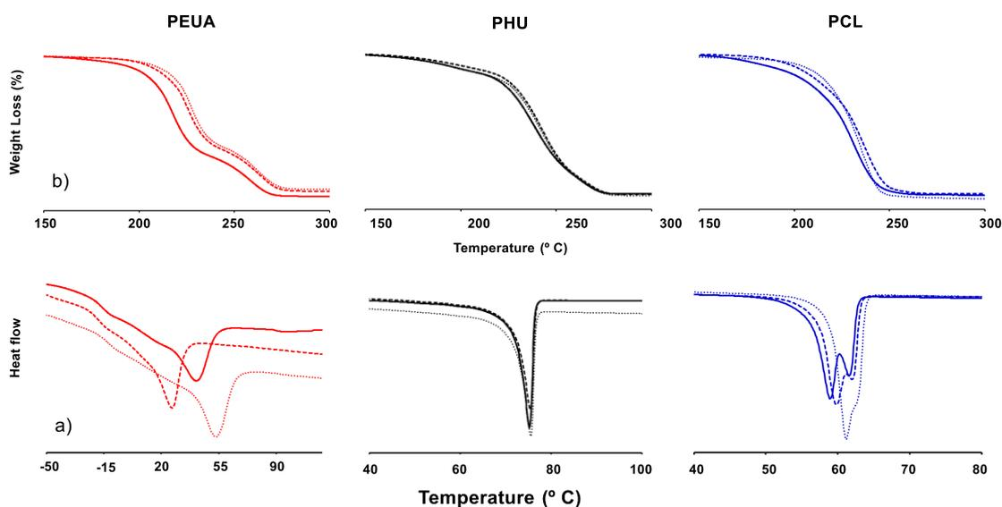
**Figure 3.** Second heating DSC (a) and TGA plots (b) of initial polyesters (—), polyesters after 10 weeks incubation at pH 2.0 at 45 °C (----) and polyester after 10 weeks incubation at pH 7.4 at 37 °C with porcine pancreas lipase (.....).
