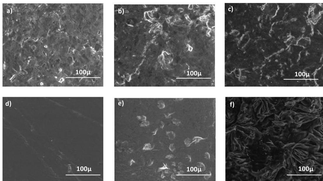
**Figure SI.5.** ESEM micrographs of a) initial PHU; b) PHU after incubation at pH 2.0 at 45 °C; c) PHU after incubation at pH 7.4 at 37 °C, d) initial PCL; e) PCL after incubation at pH 2.0 at 45 °C and f) PCL after incubation at pH 7.4 at 37 °C with porcine pancreas lipase
