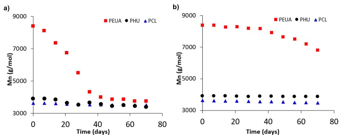
**Figure 2.** Degradation of polymers by SEC determination; a) Molecular weight at pH 2.0 at 45 °C; b) Molecular weight at pH 7.4 at 37 °C with porcine pancreas lipase.
