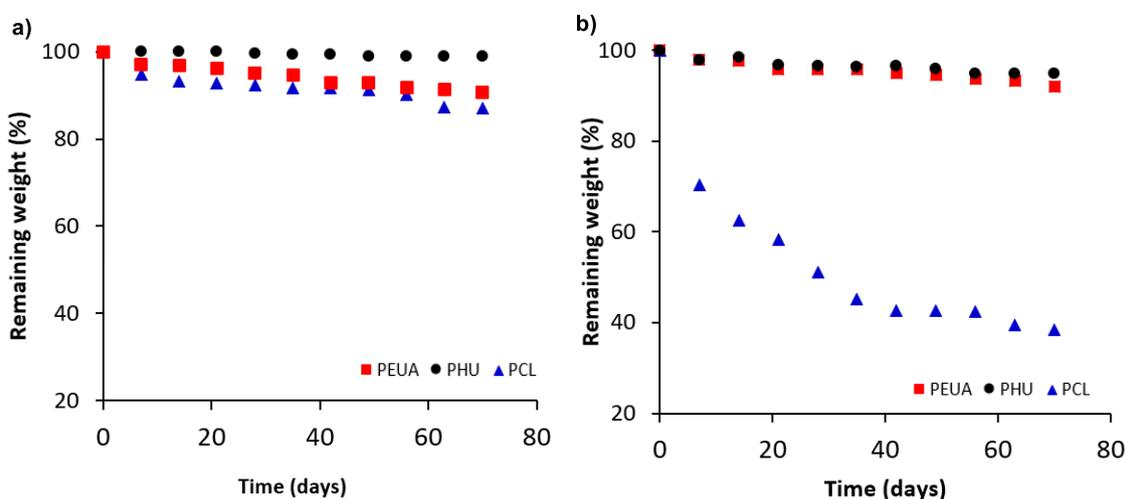
**Figure 1.** Remaining weight of polymers by measure of weight loss versus time: a) at pH 2.0 at 45 °C; b) at pH 7.4 at 37 °C with porcine pancreas lipase.
