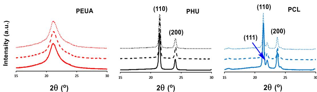
**Figure 4.** XRD patterns of initial polyesters (—), polyesters after 10 weeks incubation at pH 2.0 at 45 °C (---) and polyester after 10 weeks incubation at pH 7.4 at 37 °C with porcine pancreas lipase (.....).
