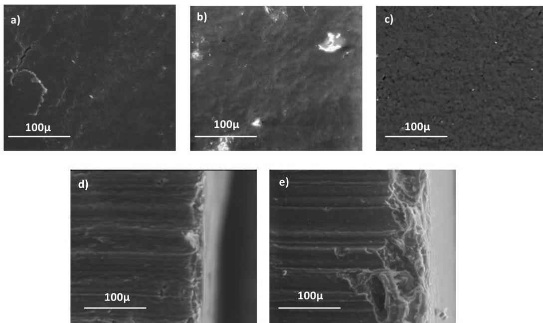
**Figure 5.** ESEM micrographs of a) initial PEUA; b) PEUA after incubation at pH 2.0 at 45 °C; c) PEUA after incubation at pH 7.4 at 37 °C with porcine pancreas lipase; d) vertical section of initial PEUA and e) vertical section of PEUA after incubation at pH 2.0 at 45 °C.
