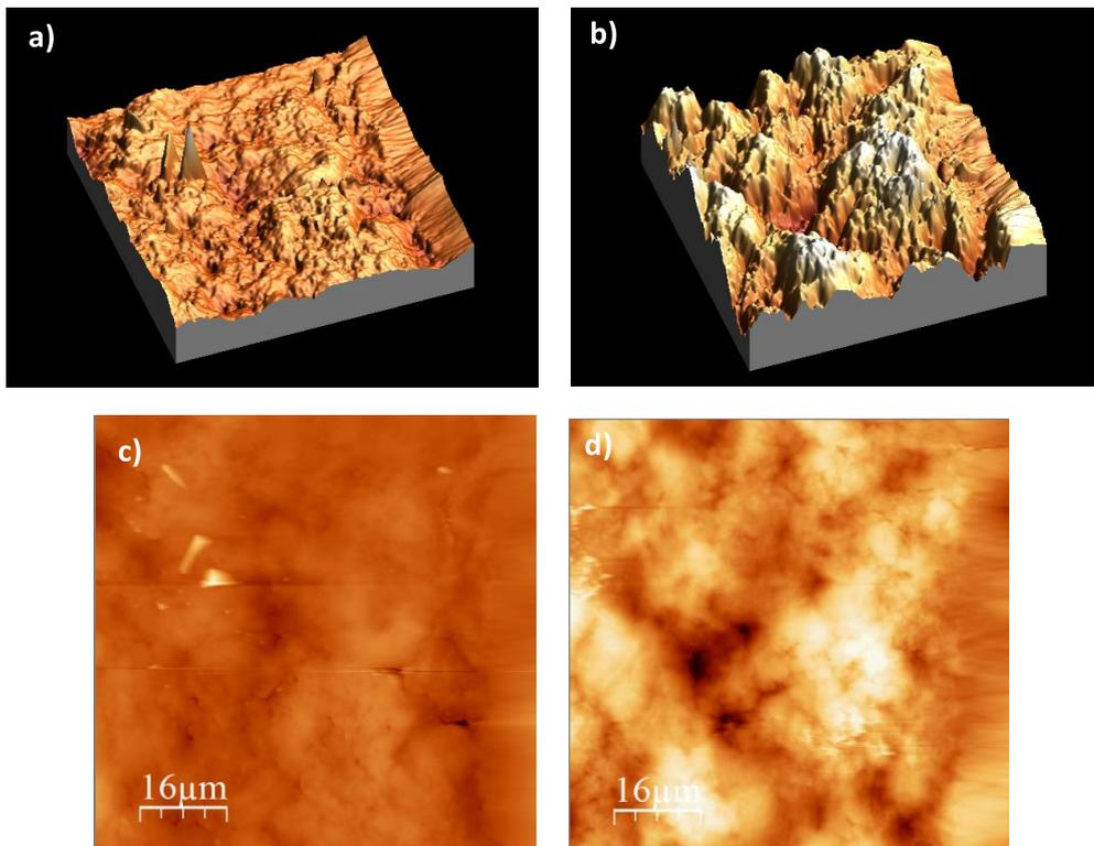
**Figure 6.** AFM images three-dimensional representation (top): a) initial PEUA; b) PEUA after incubation at pH 2.0 at 45 °C and two-dimensional representation (bottom): c) initial PEUA; d) PEUA after incubation at pH 2.0 at 45 °C.
