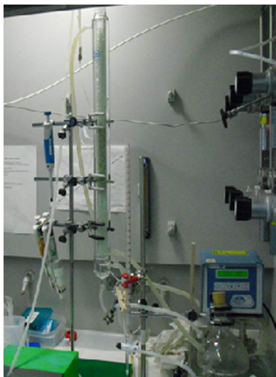
Figure 2.1. Set up of the trickle bed reactor used in this study
