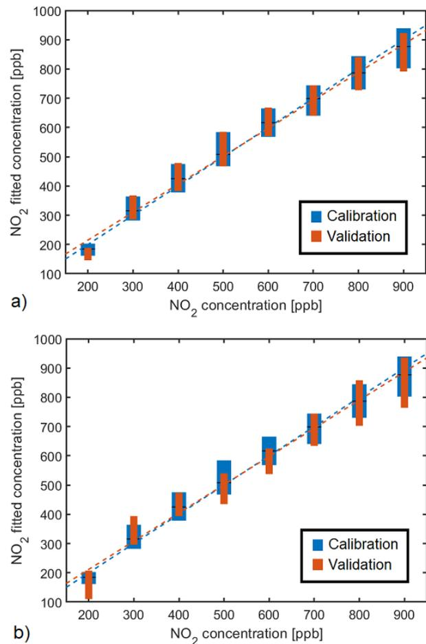
Fig. 5. PLSR calibration model and cross-validation from 9 pulses a) rates OFF and b) FFT components. Blue boxes represent the dispersion of the calibration for each concentration and orange boxes represent the validation dispersion. Black lines are the calibration mean value for each concentration. The linear calibration fit and the linear validation fit are presented in blue and orange dashed lines, respectively.
