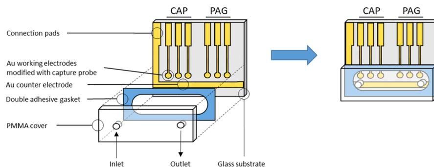
**Figure 5.** Scheme of the electrode array and the microfluidic cell.
