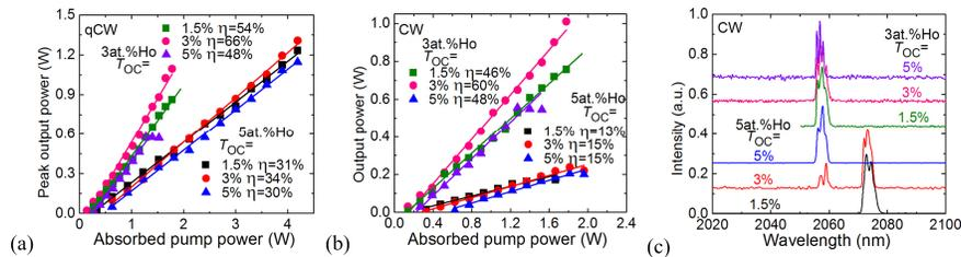
Fig. 2. (a,b) Input-output dependences for the 3 and 5 at.% Ho:KYW thin-disk lasers in quasi-CW (qCW, duty cycle 1:2) (a) and CW (b) operation modes (symbols: experimental data, lines: fits for the calculation of the slope efficiency  $\eta$ ); (c) typical laser emission spectra for the Ho:KYW thin-disk lasers for various OCs (CW regime,  $P_{abs} \sim 1.7$  W). The laser polarization is  $E \parallel N_m$ .
