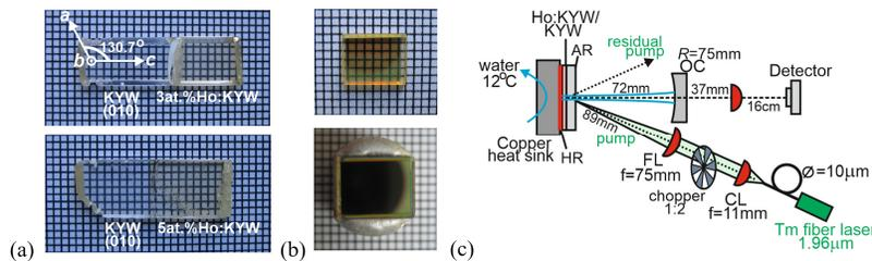
Fig. 1. (a) Photograph of the as-grown 3 and 5 at.% Ho:KYW/KYW epitaxies, their orientation with respect to the crystallographic axes (*a*, *b*, *c*); (b) cut, polished, and AR/HR coated 3 at.% Ho-doped sample (top image) soldered to a Cu heat-sink (bottom image); (c) thin-disk laser set-up: CL – collimating lens, FL – focusing lens, HR and AR – high-reflection and antireflection coatings, respectively, OC – output coupler.
