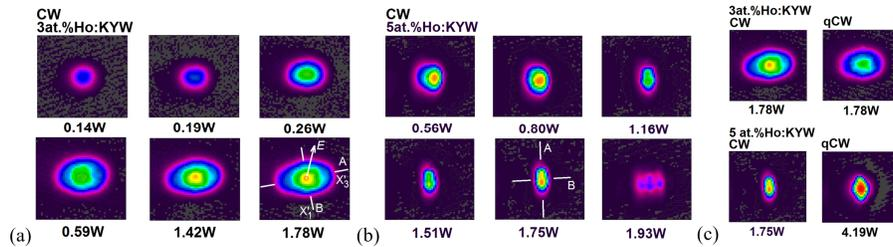
Fig. 3. (a,b) Spatial profiles of the output laser beam for the 3 at.% Ho:KYW (a) and 5 at.% Ho:KYW (b) thin-disk lasers measured at different  $P_{\text{abs}}$  as indicated by the numbers below the figures (CW regime,  $T_{\text{OC}} = 1.5\%$ ); (c) comparison of the spatial profiles of the output laser beam for the 3 and 5 at.% Ho:KYW thin-disk lasers in the CW and quasi-CW (qCW) regimes.
