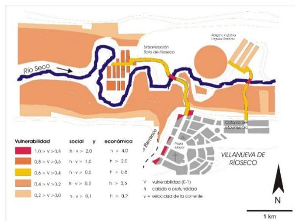
Fig. 6. Vulnerability map to flooding.
