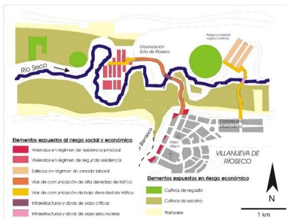
Fig. 5. Map of exposed elements to flooding.
