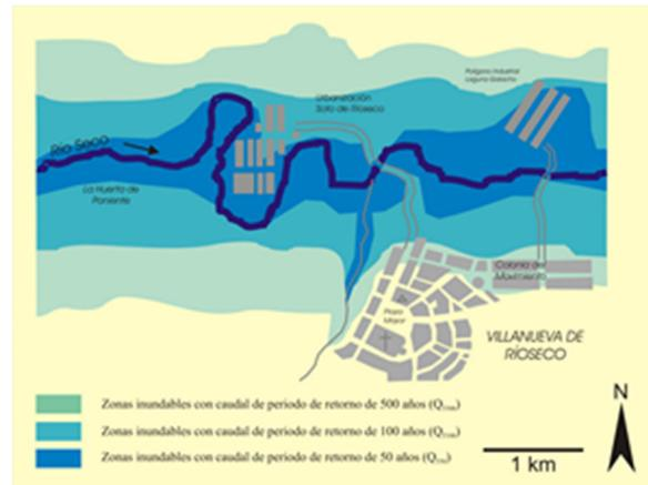
**Fig.2.** Floodable area map for discharges corresponding to different return periods.
