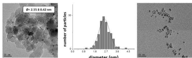
Figure 2 TEM micrographs and size distribution of nanoparticles Rh-NPs@SiO<sub>2</sub>. (20 nm scale bar)
