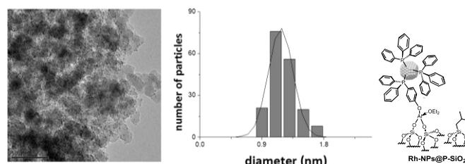
Figure 3 TEM micrograph and size distribution of nanoparticles Rh-NPs@P-SiO<sub>2</sub>, scheme of the material. (50 nm scale bar)
