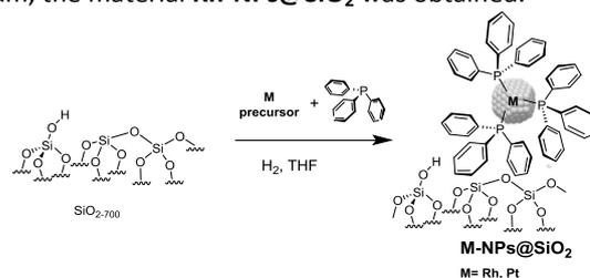
Figure 1 Scheme of the synthesis of silica supported rhodium PPh<sub>3</sub> stabilized NPs M-NPs@SiO<sub>2</sub>.
