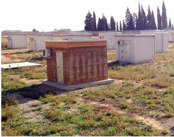
Fig. 2. Cubicles build at the testing site of University of Lleida and section showing the components of the envelope of the cubicle used for calibration [6].
