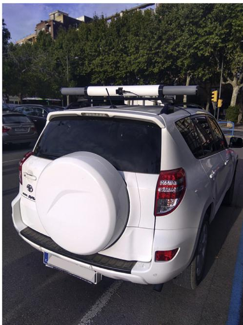
Fig. 1. Rear view of the mobile unit with the detectors installed on the roof rack.
