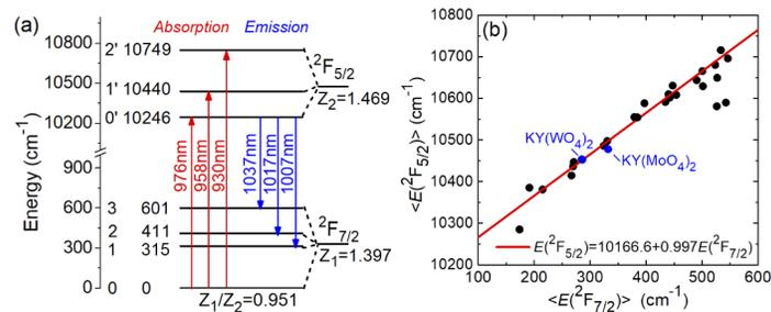
**Fig. 9.** (a) Crystal-field splitting of the  $\text{Yb}^{3+}$  ion in the  $\text{KY}(\text{MoO}_4)_2$  crystal (site symmetry:  $C_2$ ),  $Z_{1(2)}$  are the partition functions for the ground- and excited-state, respectively, arrows indicate the transitions in absorption / emission at 6 K; (b) barycenter plot [37] for the  $\text{Yb}^{3+}$  ion showing the position of  $\text{Yb}:\text{KY}(\text{WO}_4)_2$  and  $\text{Yb}:\text{KY}(\text{MoO}_4)_2$  crystals (blue circles).
