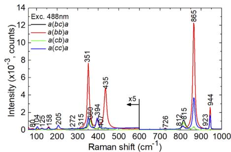
**Fig. 5.** RT Raman spectra of the 3 at.% Yb:KY(MoO<sub>4</sub>)<sub>2</sub> crystal for the *a(mn)a*, *m*, *n* = *b*, *c* geometries (Porto's notations),  $\lambda_{\text{exc}} = 488$  nm, *numbers* indicate the peak frequencies in cm<sup>-1</sup>.
