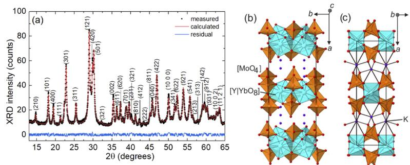
**Fig. 2.** (a) Rietveld analysis of the RT X-ray powder diffraction (XRD) pattern of a 3 at.% Yb:KY(MoO<sub>4</sub>)<sub>2</sub> crystal, the numbers denote the Miller's indices (*hkl*) for the sp. gr. *Pbna*; (b,c) Illustration of the layered structure of the Yb:KY(MoO<sub>4</sub>)<sub>2</sub> crystal: (b) three-dimensional view, (c) a projection of the *a-c* plane. Black rectangle denotes the unit-cell.
