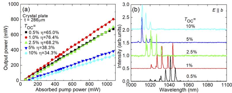
**Fig. 11.** Diode-pumped Yb:KY(MoO<sub>4</sub>)<sub>2</sub> cleaved crystal-plate microchip laser: (a) input-output dependences,  $\eta$  – slope efficiency; (b) typical laser emission spectra measured at  $P_{\text{abs}} = 1.0 \text{ W}$ . The laser polarization is  $E \parallel b$ .
