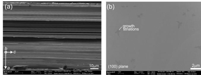
**Fig. 4.** Scanning Electron Microscope (SEM) images of a cleaved single-crystal plate of 3 at.% Yb:KY(MoO<sub>4</sub>)<sub>2</sub>: (a) the fracture edge of the plate running along the *c*-axis, the *a*-axis is vertical; (b) the plate surface parallel to the (100) plane showing flower-like defects.
