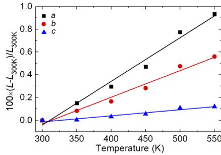
**Fig. 3.** Relative thermal evolution of the unit cell parameters of 3 at.% Yb:KY(MoO<sub>4</sub>)<sub>2</sub> with the temperature up to 550 K.
