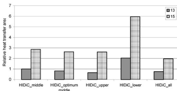
Fig. 6 – Heat transfer area relative to the *HIDiC(15)\_middle*
