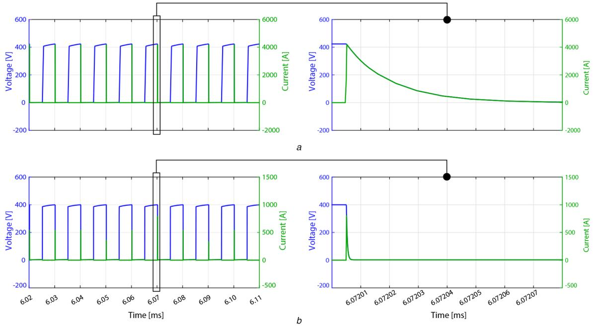
**Fig. 10** Simulated results of current and voltage across the SW  $Q_2$  for boost mode using LTSpice
