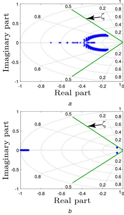
**Fig. 5** Roots of the characteristic polynomial of the PS2 converter
