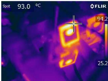
**Fig. 11** Thermal image of the half-bridge MOSFET boost side
