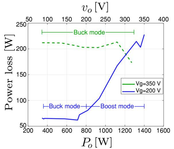
**Fig. 16** Total power loss for PS1
