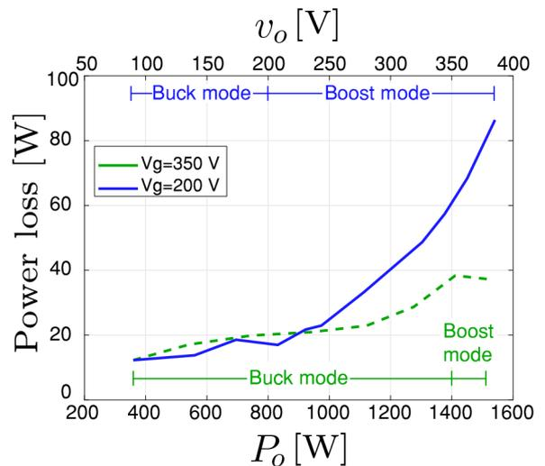
**Fig. 17** Total power loss for PS2
