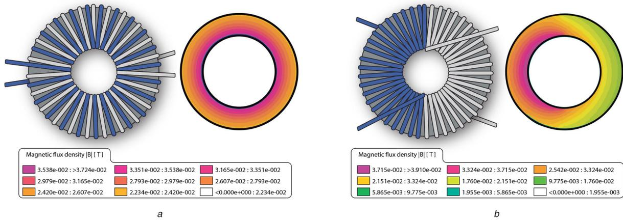
**Fig. 9** Flux density map of the coupled inductors modelled using FEMM
