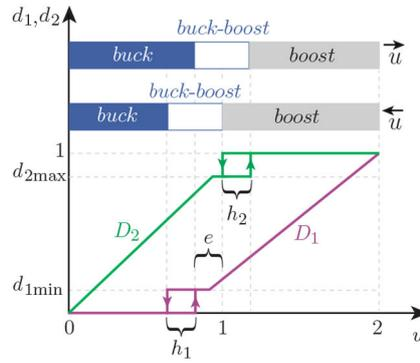
Fig. 3 Scheme of the hysteretic transition method
