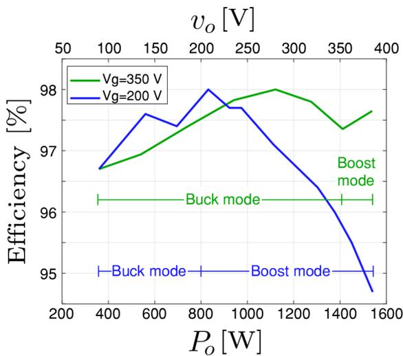
**Fig. 15** Energy conversion efficiency for two different values of  $V_g$  (200 V and 350 V) with a  $I_L = 4$  A as a function of the output power  $P_o$  for PS2
