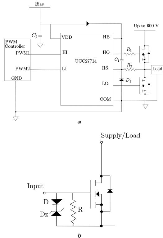
**Fig. 8** Diagram of (a) Circuit schematic driver, (b) Transient voltage MOSFET protection
