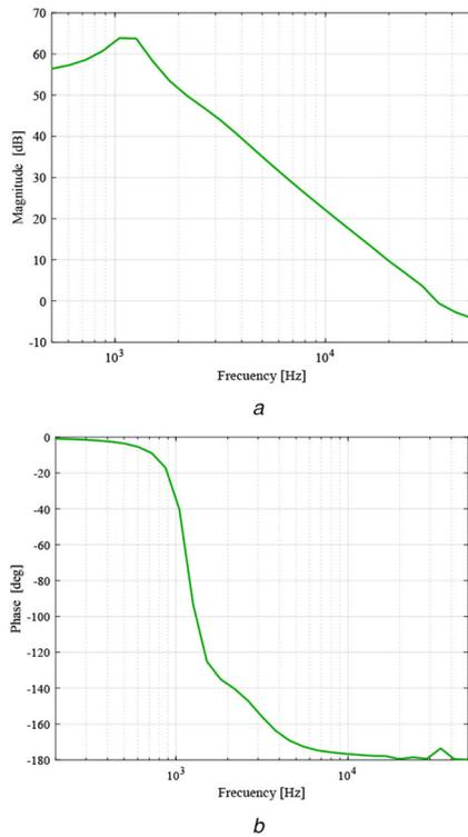
**Fig. 6** Frequency response of the small-signal control-to-output transfer function. Simulation of the switched model using PSIM in boost mode (a) Magnitude [dB], (b) Phase [deg]
