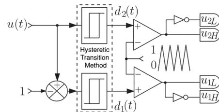
**Fig. 2** Diagram of switch signals generation
