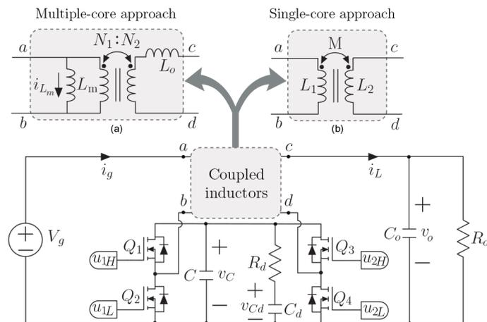
**Fig. 1** Schemes of the buck–boost power stage
