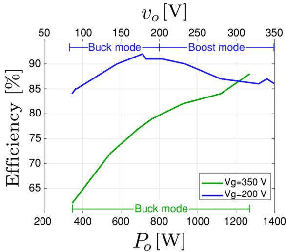
**Fig. 14** Energy conversion efficiency for two different values of  $V_g$  (200 V and 350 V) with a  $I_L = 4$  A as a function of the output power  $P_o$  for PS1
