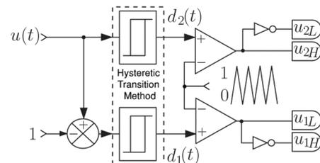
**Fig. 2** Diagram of switch signals generation
