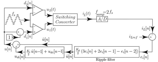
**Fig. 12** Schematic diagram of the two-loop control using MACC method
