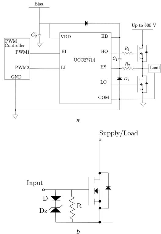
**Fig. 8** Diagram of (a) Circuit schematic driver, (b) Transient voltage MOSFET protection
