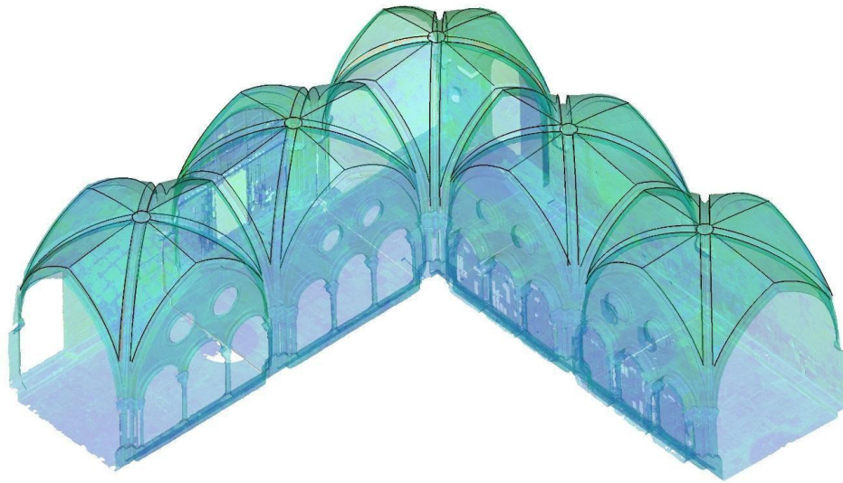
Figure 4. Mesh of the north corner of the cloister of the Cathedral of Tarragona.
