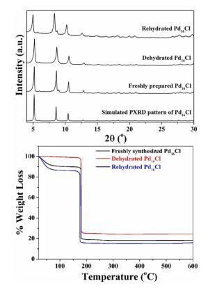
*Figure 3.* (top) PXRD patterns and (bottom) TGA curves of freshly prepared, dehydrated, and rehydrated compound **Pd<sub>16</sub>Cl**.
