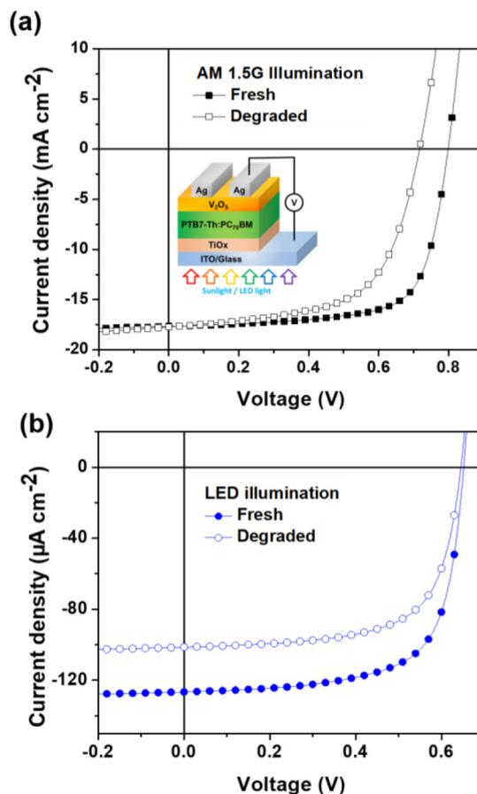
**FIGURE 1.** Illuminated current density-voltage ( $J - V$ ) characteristics of fresh (solid symbol) and degraded (open symbol) cells exposed under (a) AM 1.5G and (b) 1000 lux LED 2700 K irradiation. The light intensity of AM 1.5G spectrum is  $100 \text{ mW cm}^{-2}$  and 1000 lux LED 2700 K spectrum is  $0.35 \text{ mW cm}^{-2}$ . The inset figure is the architecture of inverted PTB7-Th:PC<sub>70</sub>BM-based devices fabricated in this study.
