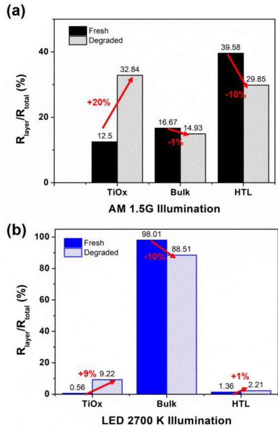
**FIGURE 5.** The percentage contribution of each layer resistance to the total resistance of the cells for fresh and degraded devices photodegraded under (a) standard AM 1.5G and (b) 1000 lux LED 2700K irradiation. The values were extracted by modeling the IS measurements at open-circuit conditions.
