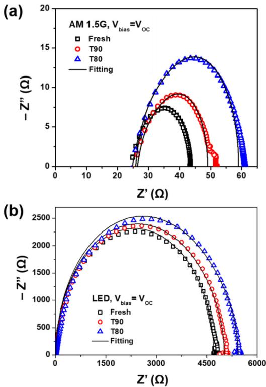
**FIGURE 4.** Cole-Cole plots at open-circuit voltage bias over aging time of PTB7-Th:PC<sub>70</sub>BM-based devices under (a) AM 1.5G and (b) 1000 lux LED illumination. The experimental results were fitted using the 3RC circuit model (solid lines).
