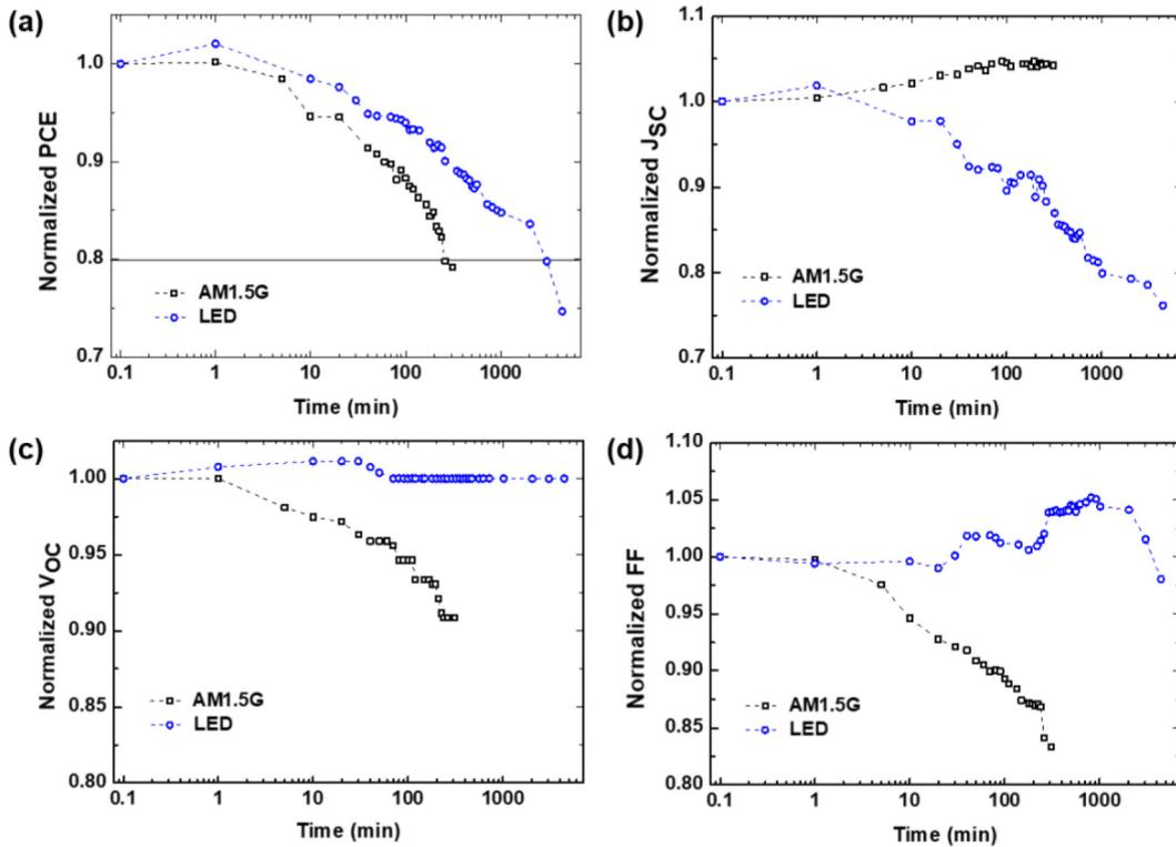
**FIGURE 2.** Normalized device performance parameters (a) PCE, (b)  $J_{SC}$ , (c)  $V_{OC}$ , and (d) FF of inverted PTB7-Th:PC<sub>70</sub>BM-based device under two light sources exposure: AM 1.5G solar simulator (black squares) and 1000 lux LED lamp (blue circle).
