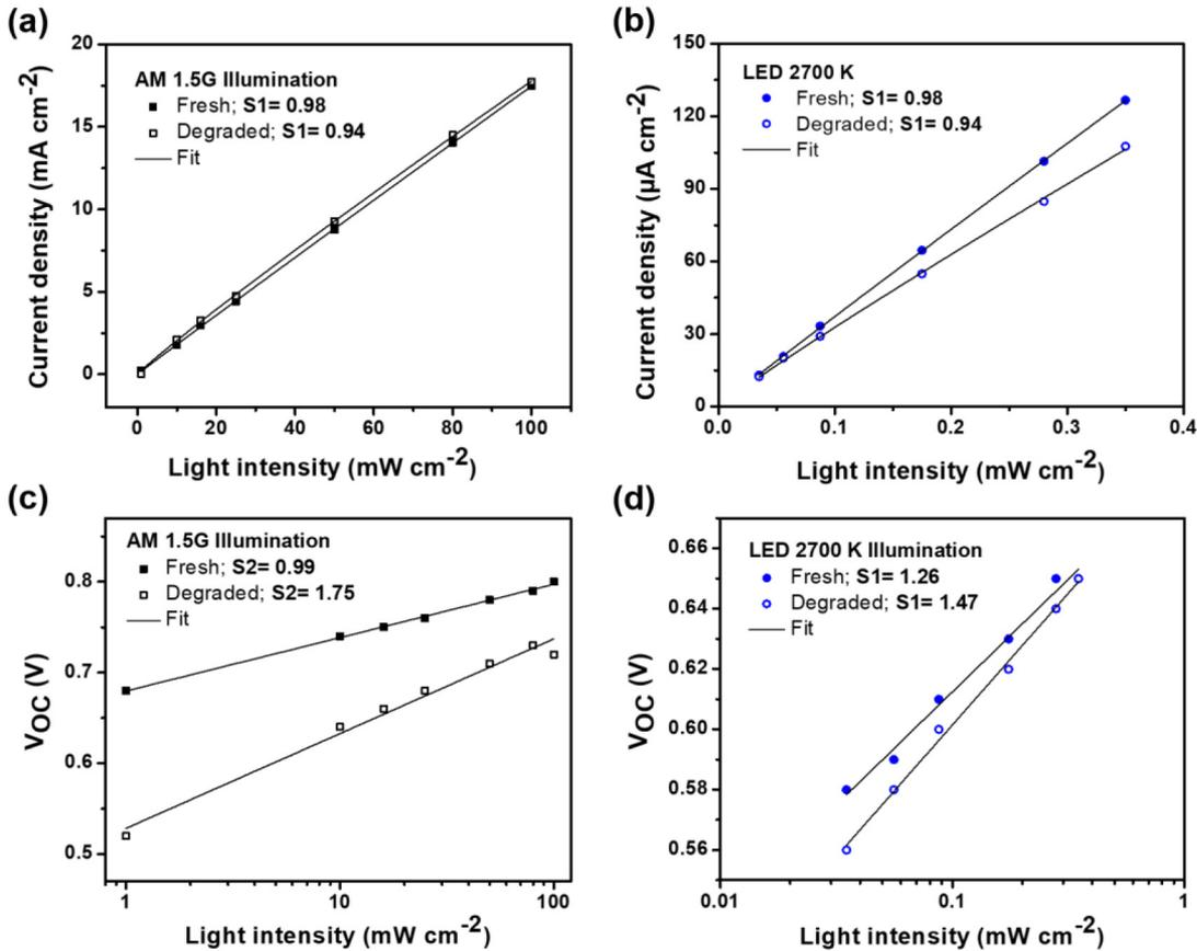
**FIGURE 3.** (a,b)  $J_{SC}$  and (c,d)  $V_{OC}$  dependence on light intensity over aging time of inverted PTB7-Th:PC<sub>70</sub>BM-based device under (a,c) AM 1.5G and (b) 1000 lux LED light illumination. All measurements were carried out in an inert atmosphere.
