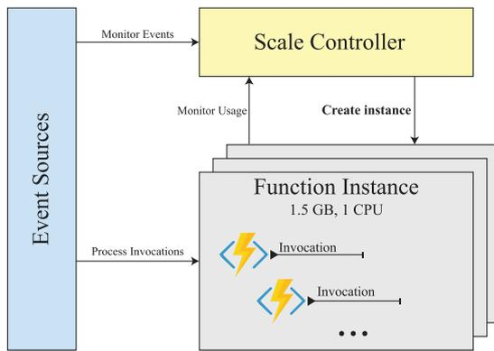
Fig. 3. Azure Functions architecture.
