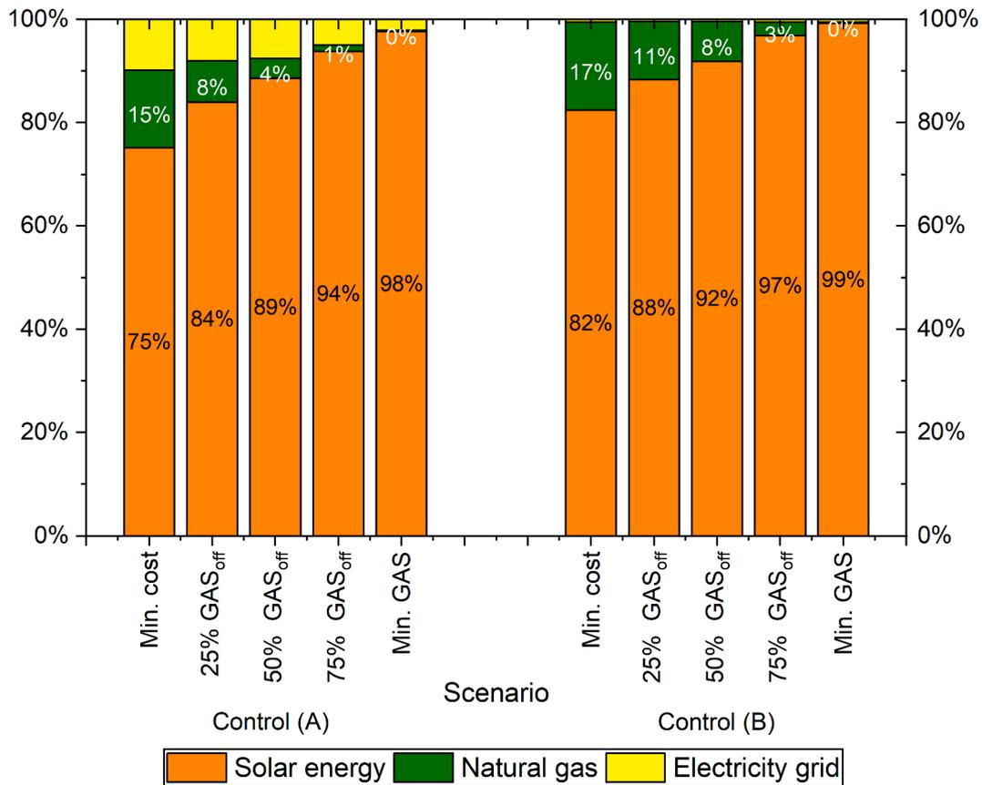
Fig. 5. The share of technologies for the optimal Pareto solutions of the HP integrated with SDHS under control strategy (A) and (B).
