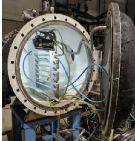
Figure 1. Falling film absorber for water/LiBr mixture
