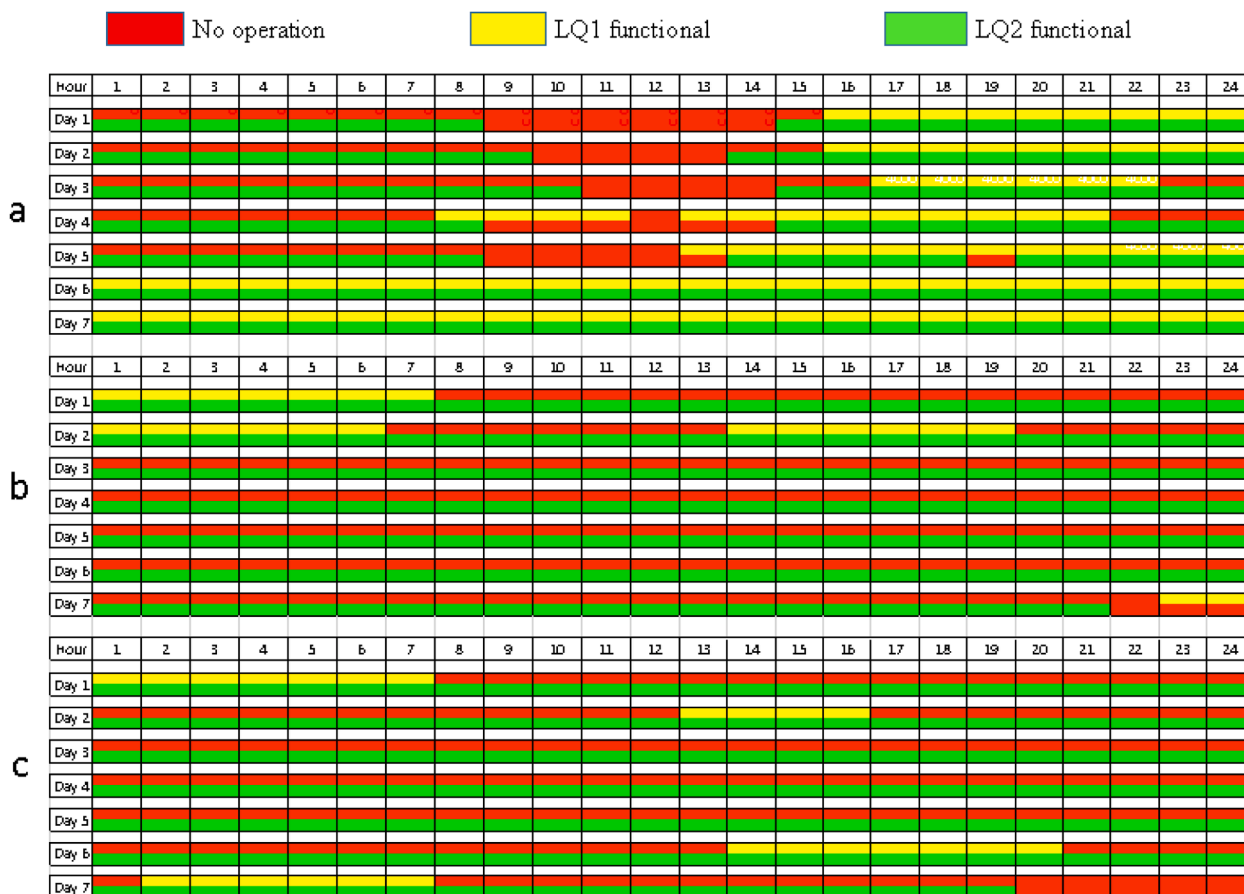
Fig. 9. Optimal scheduling schemes for (a) deterministic forecast of electricity prices (b) scenario corresponding to the lower quartile the profit distribution (c) scenario corresponding to the upper quartile of the profit distribution.
