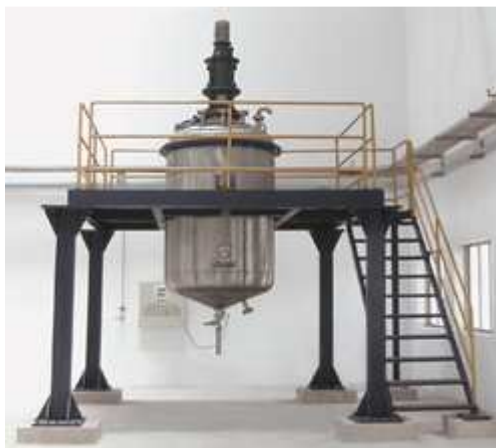
Figure 4.4. Representation of the structure in agitation tank.
