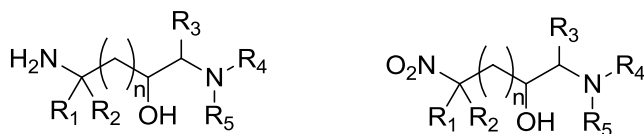
Figure 1.4 Amino alcohol compounds that are useful as neutralizing agents for aqueous based paints and coatings.
