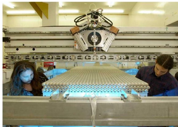
Figure 2.18: Left: Drift Chamber. The drift cell is defined at one end by a high voltage electrode and at the other end by the anode of a simple proportional counter. To signal the arrival of a particle, a scintillation counter is placed before and after the chamber. A particle traversing the chamber and scintillator, now, liberates electrons in the gas which then begin drifting towards the anode. At the same time, the fast signal from the scintillator starts a timer. The signal created at the anode as the drifting electrons arrive then stops the timer to yield the drift time. Picture taken from [29]. Right: Working on the assembly of MDT tubes [13].
