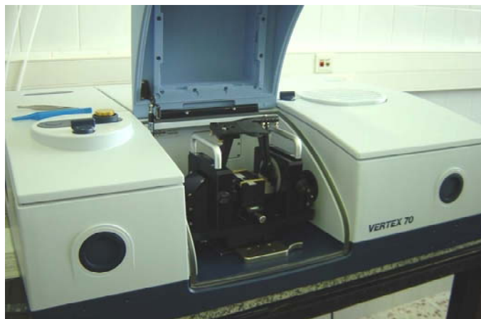
Fig. 5.14. Photograph of the FTIR spectrometer Bruker Vertex 70 used for the measurement of the porous silicon layers. The setup for the measurement of the reflectivity spectrum is placed.
