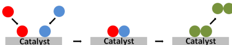
Figure 1.2: Scheme of a catalytic process through the Langmuir-Hinshelwood mechanism.
