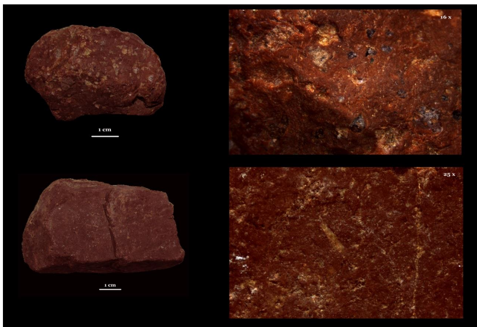
Fig. 3.29. Stereomicroscope observation of the samples collected along the Sessera river. In the aphyric matrix are well visible quartz and feldspar phenocrysts.
