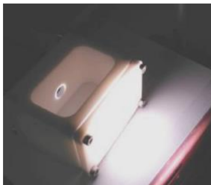
Figure S10. Photography of the custom-made Teflon cell used for the (photo)electrochemical experiments (adapted from 2 ).
