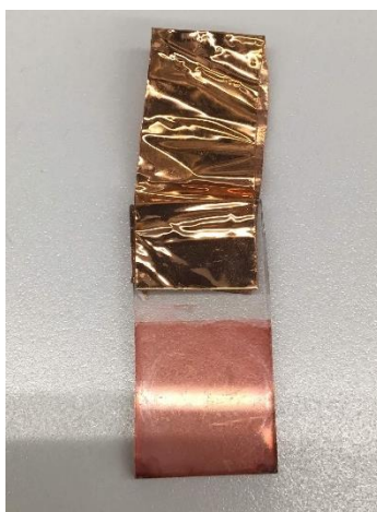
Figure S1. Photography of PDI@ATO@FTO after preparation.
