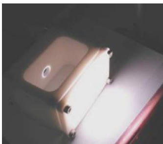
Figure S4. Photography of the custom-made Teflon cell used for the (photo)electrochemical experiments (adapted from 3 ).
