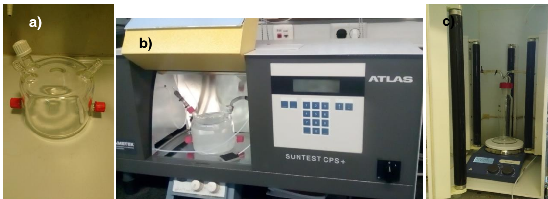
Picture 1. (a) Reactor for SSL-system, (b) solar simulated chamber and (c) reactor for UVA-system and UV box
