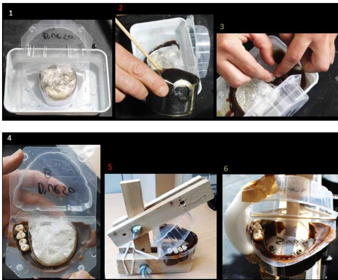
Fig. 27: Creation of experimental mandible. 1: dentist plastic box inside cold water; 2: gum reconstruction with glue (30% resin/70% beeswax); 3: placement of teeth; 4: mandible with four third molars with caries in sequence; 5: blocking of mandible open; 6: cheek of mandible.
