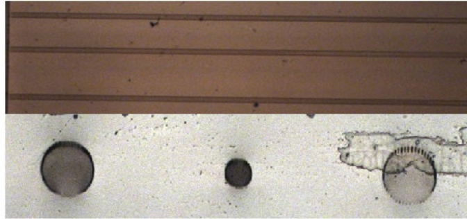
Figure 3. Top and frontal confocal microscopy of three funnel shaped waveguide channels with different radius ( 30 μm, 15 μm and 30 μm )
