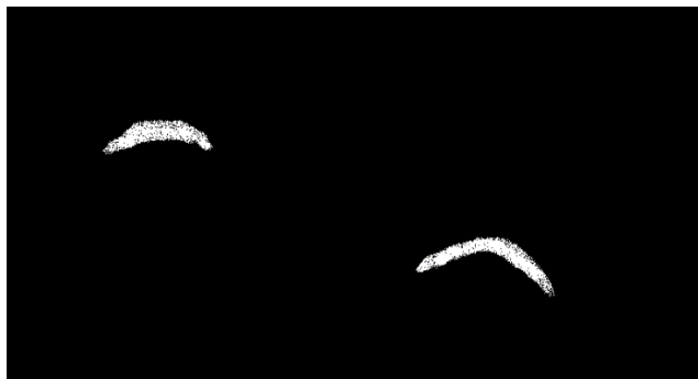
Figure 2. Camera binary image of two fingers interacting with the laser beam.
