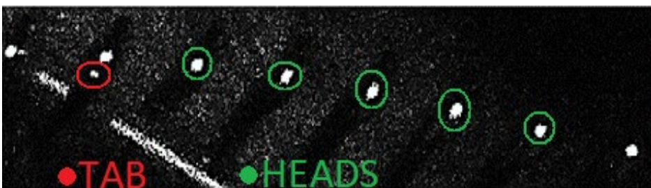
Figure 34. image captured by the ultra-fast camera. In green you can see white points that represent the heads of the pins and in red a smaller white point that are the tabs can be seen.
