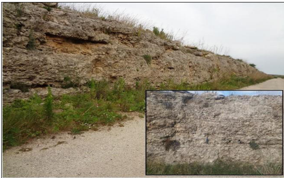
Figure 3.2-4: Road cut of calcarenite deposits of Grande Terrazzo Superiore (G.T.S). In square frontal view of calcarenites, in this point sample, Calc\2 was sampled
