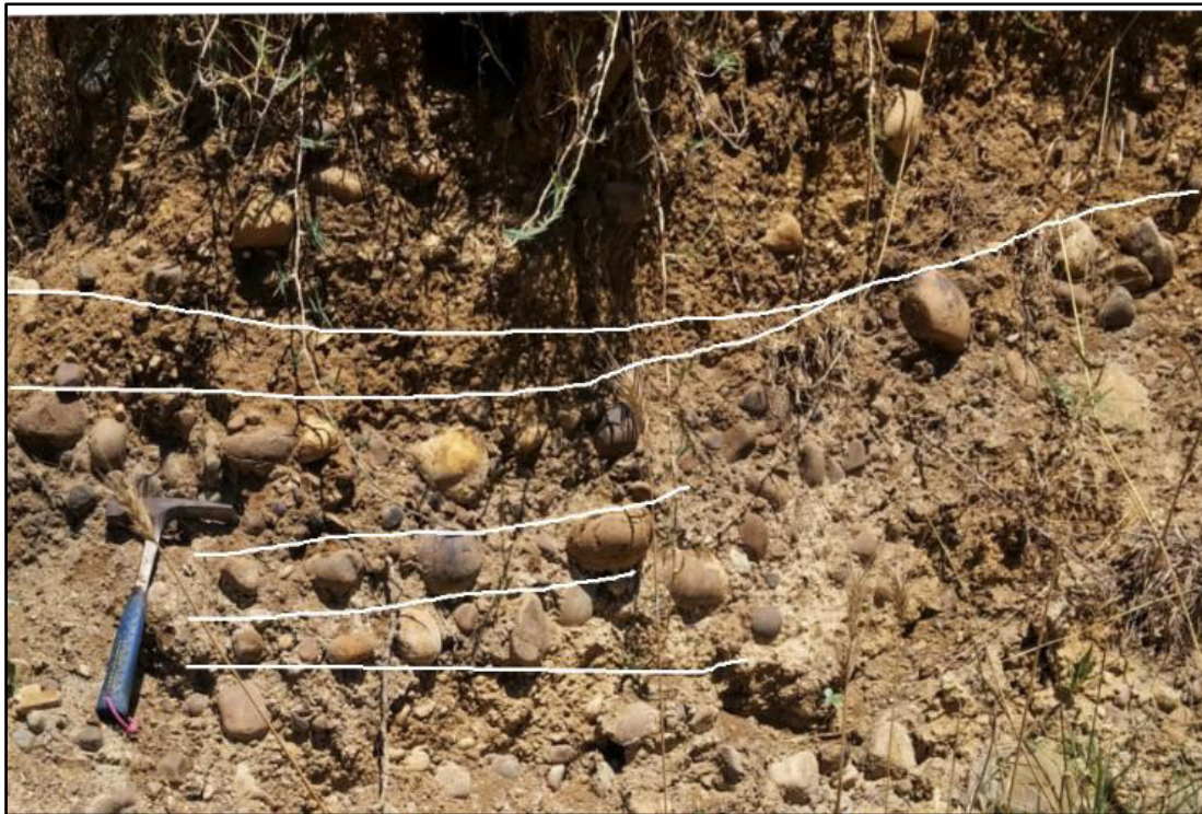
Figure 3.4-7: conglomerate layers of the S7\M5 outcrop, white line shows the plane-parallel orientation.
