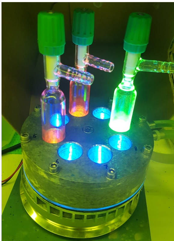
FIGURE 4.4. Photoreactor setup with 8 parallel reactors photographed through a 450 nm notch filter.
