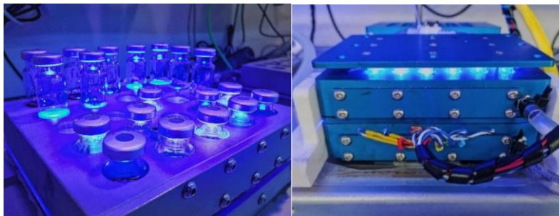
Figure 3. 10. In house developed parallel photoreactors with (left) 25 positions for vials of 10 or 21 mL and (right) with 48 positions for vials of 1 mL.
