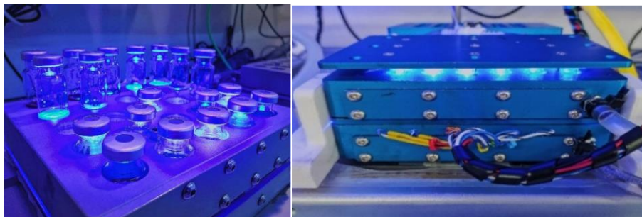
Figure 4. 4. In house developed parallel photoreactors with (left) 25 positions for vials of 10 or 21 mL and (right) with 48 positions for vials of 1 mL.
