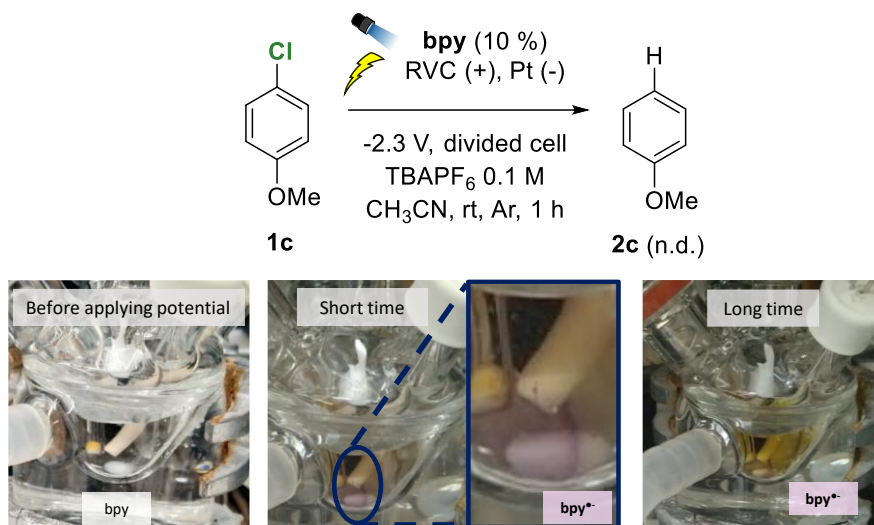
Figure 5.27. Electrocatalytic dechlorination using bpy as a catalyst in acetonitrile. Pictures of a non-irradiated experiment, a purple gradient precedent from the reduction in the electrode foam, but it quickly vanishes in bulk, which gets more and more yellow with time, consistent with the accumulation of 3-aminocrotonitrile.
