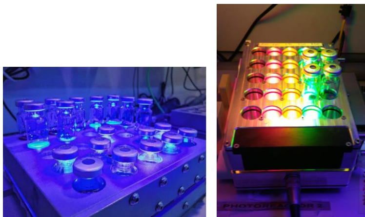
Figure 5. 29. In-house developed parallel photoreactors with 25 positions for vials of 10 or 21 ml.
