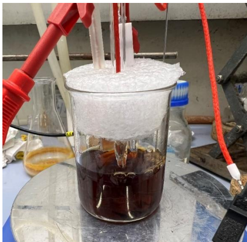
Figure 25: Image of the set-up used for the electropolymerization of the molecular complexes onto the electrode.
