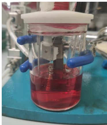
Figure 33: Image of the set-up used to perform the molecular complexes electropolymerization onto the semiconductor
