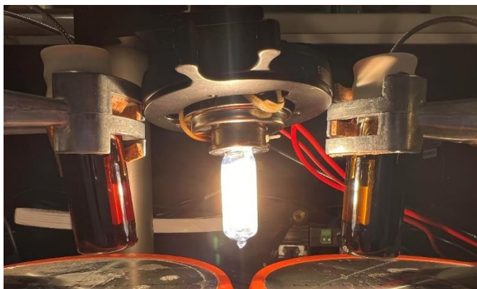
Figure 27: Image of the set-up used to perform the immobilization of the Ru complexes onto the electrode by thiol-ene click reaction.
