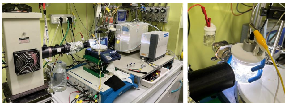
Figure 30: Image of the set-up used to perform the CO 2 reduction tests
