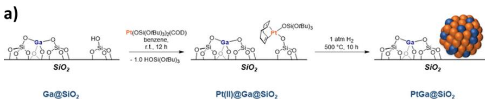
Scheme 5.1. (a) Synthetic procedure employed for PtGa alloyed NPs supported on Ga-doped silica using SOMC approach. 7
