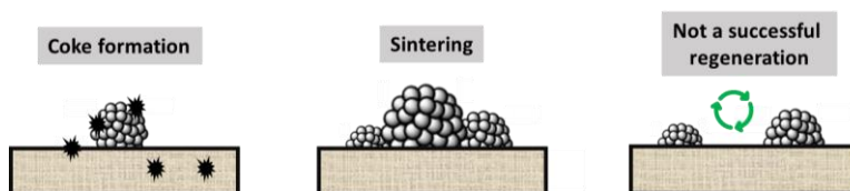
Figure 1.7. Main mechanisms of deactivation for metal-based and metal-oxide-based catalysts.
