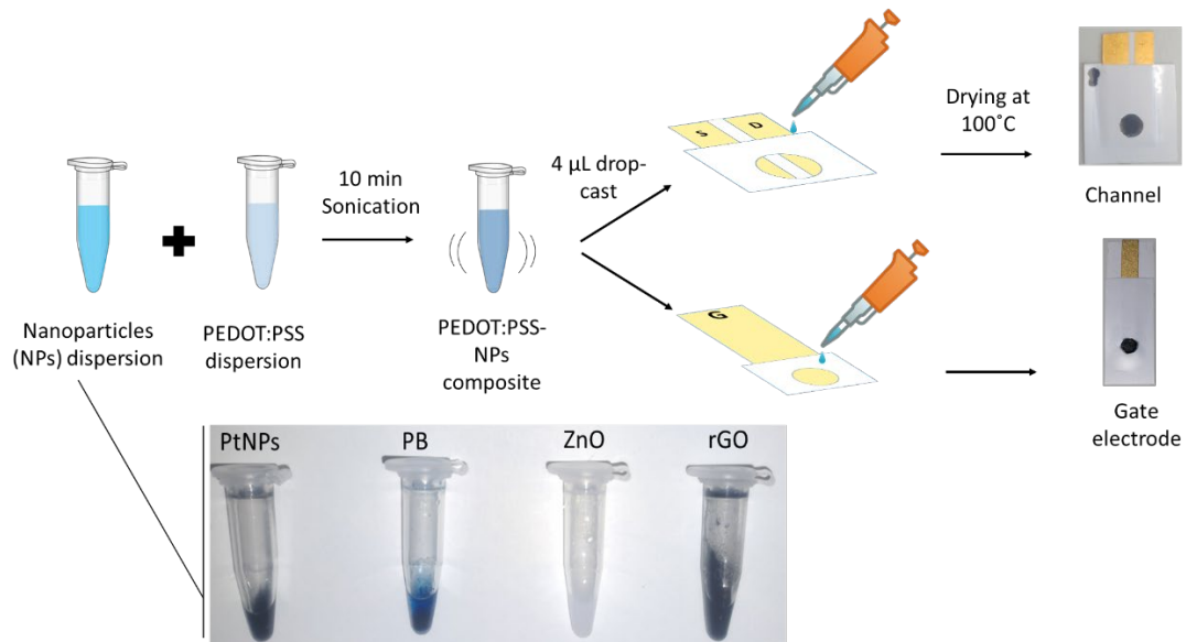
Figure 6.1. Description of the fabrication steps of the sensors, and the nanoparticles suspended in ethanol.
