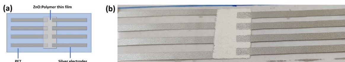
Figure 7.4 (a): Schematic of ZnO PENG, (b): ZnO-PVA screen printed thin film with commercial silver ink busbar electrodes on PET substrate
