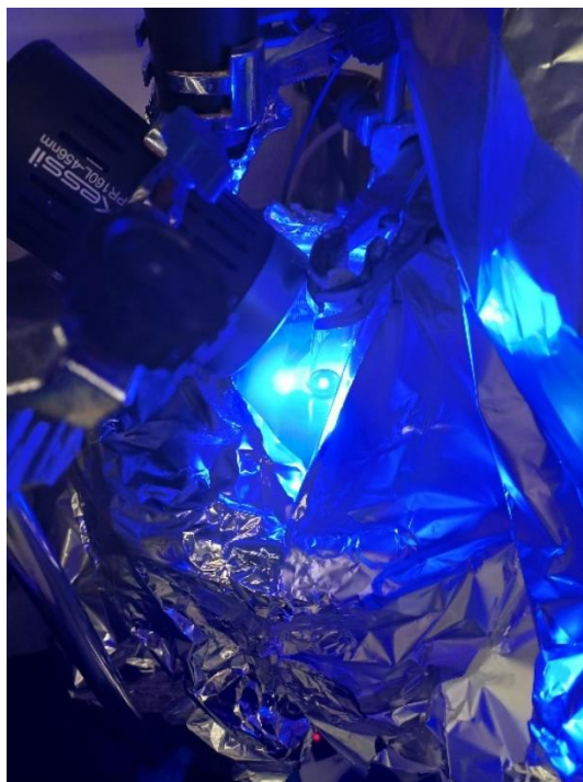
Figure 3.29. Set-up for the conjugate cyanation of octenal 1a using a Kessil lamp (456 nm, maximal intensity). The vial was placed in a toluene bath which was externally cooled to 5 °C by a cryostat (Thermo Fisher Scientific - EK90 Immersion Cooler). Distance from the Kessil lamp to the bottom of the vial was approximately 5 cm.
