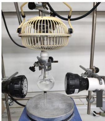
Figure 4.22. Setup for the gram-scale experiment using two EvoluChem lamps emitting at 405 nm.
