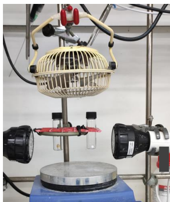
Figure 4.21. Reaction setup using EvoluChem lamps emitting at 405 nm
