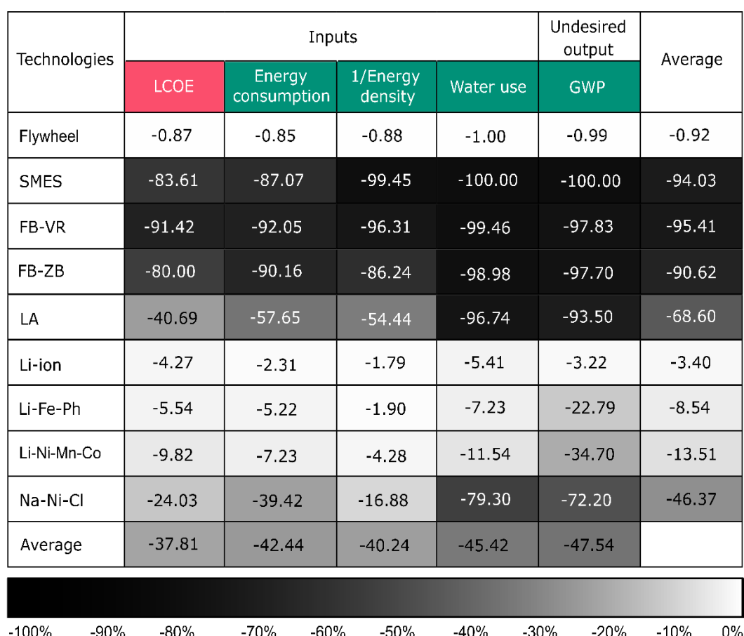
Figure 6. Improvement targets for inefficient technologies of fast-response energy storage cluster under uncertainty (%). All the indicators: demanded reduction. LCOE: Levelized cost of energy. GWP: Global warming potential.
