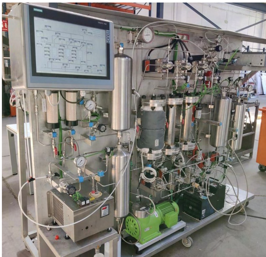
Figure 3.12: Post-combustion CO 2 capture pilot plant using VSA with TAMOF-1.
