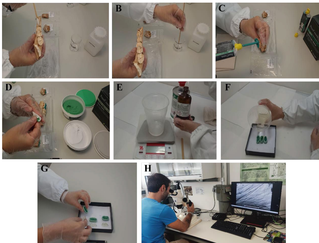
Figure 21. Different steps of the dental microwear protocol for cleaning, moulding, and casting at Biomarkers Laboratory (IPHES-CERCA; Tarragona, Spain). See the video by Martínez-Polanco et al. (2021) for more details.
