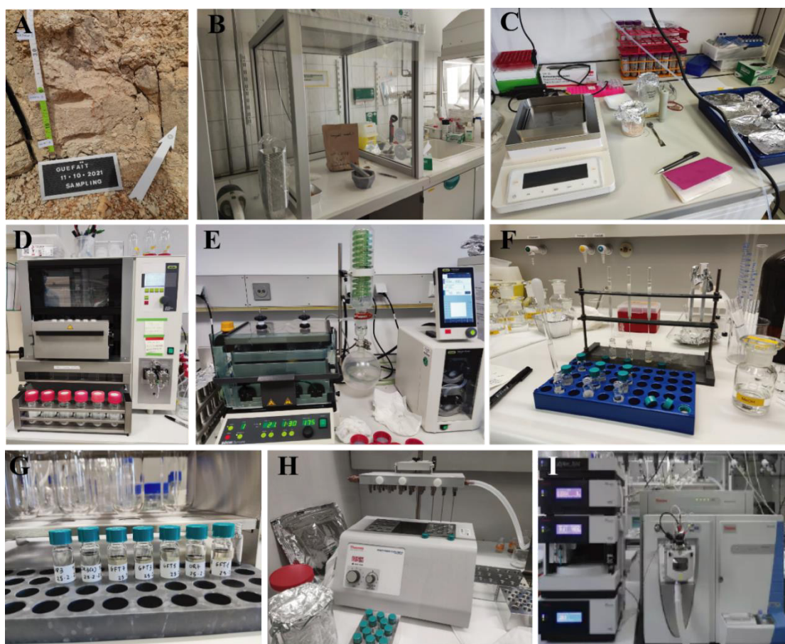
Figure 23. Protocol for plant wax biomarkers analysis at Max Planck Institute of Geoanthropology (Jena, Germany). A , Sampling of the GFT-4.2 sequence. B , Homogenisation of sediments using a mortar. C , Weighing of samples for analysis. D , Introduction of samples into the Büchi Speed Extractor E-916. E ,
