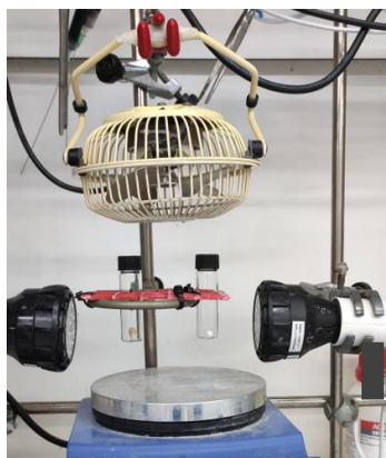
Figure 3.22. Reaction setup using EvoluChem lamps emitting at 405 nm.
