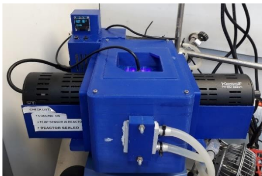
Figure 2.32. Reaction setup using a 3D-printed photoreactor under illumination at 390 nm by two Kessil lamps.
