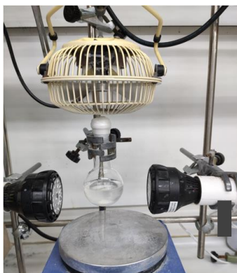
Figure 3.23. Setup for the gram-scale experiment using two EvoluChem lamps emitting at 405 nm.
