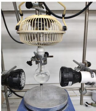
Figure 2.33. Setup for the gram-scale experiment using two EvoluChem lamps emitting at 405 nm.
