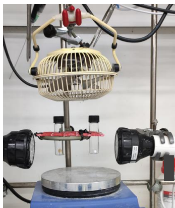
Figure 4.19. Reaction setup using EvoluChem lamps emitting at 405 nm.
