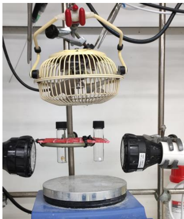
Figure 2.31. Reaction setup using EvoluChem lamps emitting at 405 nm
