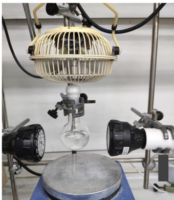
Figure 4.20. Setup for the gram-scale experiment using two EvoluChem lamps emitting at 405 nm.
