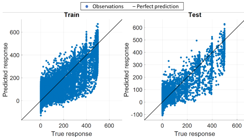
Fig. S9: Prediction chart of nitrogen dioxide removing features related to humidity and temperature. (left) train data: RMSE = 43.62 ppb, R^2 = 0.85 . (right) test data: RMSE = 50.47 ppb, R^2 = 0.81 .
