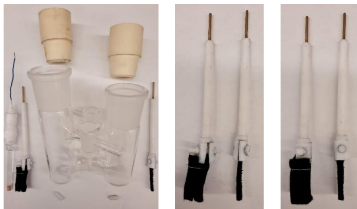
Figure 2.12 Pictures of the H electrolytic cell and the Carbon felt electrodes.
