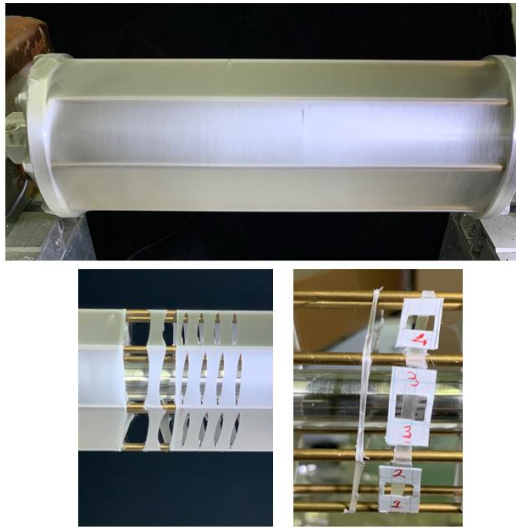
Figure 4.7. Aligned fibers collected on a wire drum and sample preparation.
