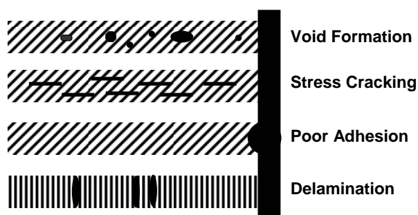
Figure 1.3. Typical polymer shrinkage problems.
