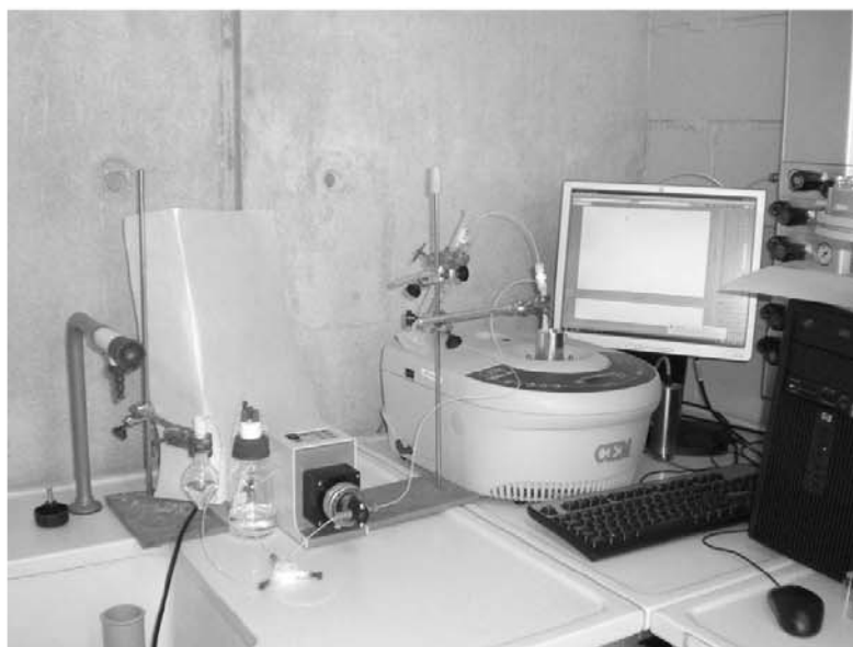
Figure 3. Continuous flow system used in the allylic amination of S1 with benzylamine.
