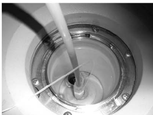
Figure 4. Detail of the teflon tube containing the polymer-supported catalyst in the microwave cavity.
